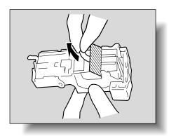
6 Insert the refilled staple cartridge holder until it locks into place.
